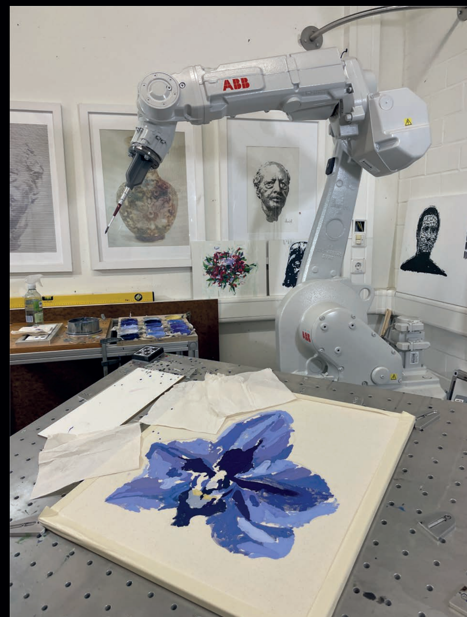
The E-David robot painting a work of Greta Louw, using image-abstraction technologies developed at Konstanz University.
