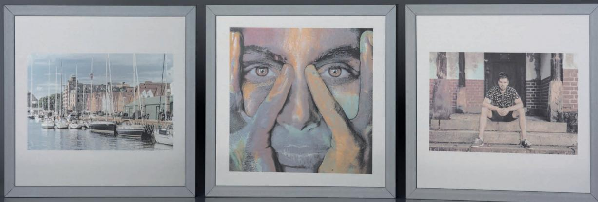
The Max Planck project "Oraclase" has developed an innovative laser production method that enables the creation of detailed, colorful images on metallic surfaces. At the heart of the approach is a novel AI-based inverse method for computing optimal process parameters, which can be used in a variety of applications such as "Color Laser Marking".
