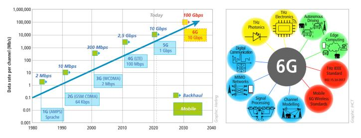
Left: Rapid development of mobile phone generations - a quantum leap in data transmission rates every ten years. Right: 6G technology requires close cooperation between different disciplines: electronic and photonic hardware development (yellow), system sciences (blue), application development (green) and standardisation organisations (red).
