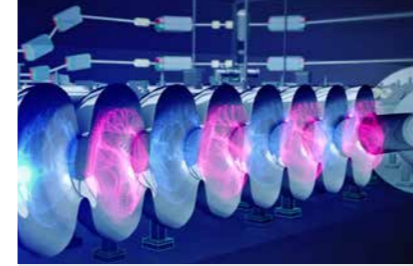
Cover: Niels Paul Bethe/PRISMA+ An inside view of a cryomodule, which is at the heart of MESA, a superconducting electron accelerator that will be used on completion for basic research in particle physics.
