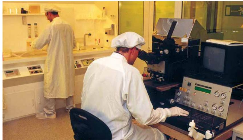
Structural transfer by means of optical lithography, under yellow light in the clean room.
