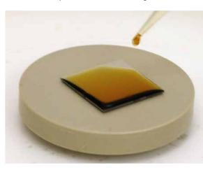
.. are applied to the wafer with a pipette prior to centrifugation.
