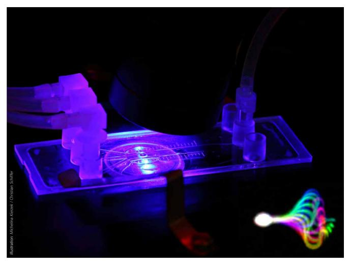
To understand navigation of freely moving sperm, they are observed under the microscope inside shallow glass capillaries with a high-speed camera. A sequence of successive, aligned, superimposed, and color-coded images allows the flagellar beating pattern to be visualised (bottom right).
