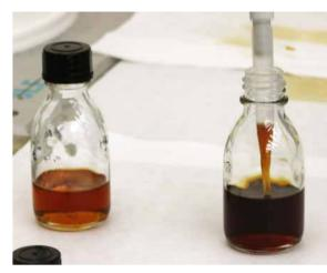
Solutions of yttrium-doped hafnium oxide (left) and undoped zirconium oxide (right) ...
