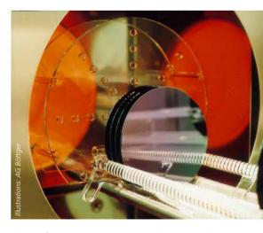
The wafers then undergo crystallisation in the diffusion furnace.
