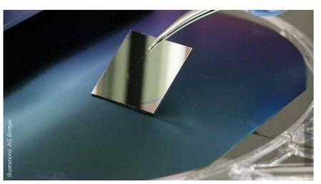
Placing a coated wafer in a quick-heating furnace for crystallisation.
