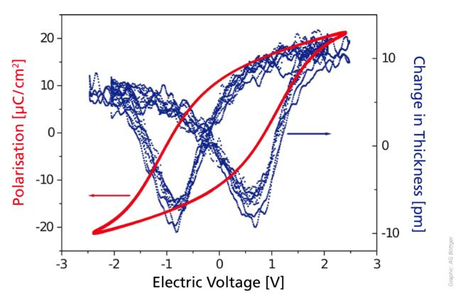
The striking butterfly shape of the electromechanical stress-strain curve for a silicon-doped hafnium oxide layer around 10 nm thick. By using a double-beam laser interferometer, it is possible to resolve changes in thickness of less than 1 picometre (1 billion picometres make 1 millimetre).
