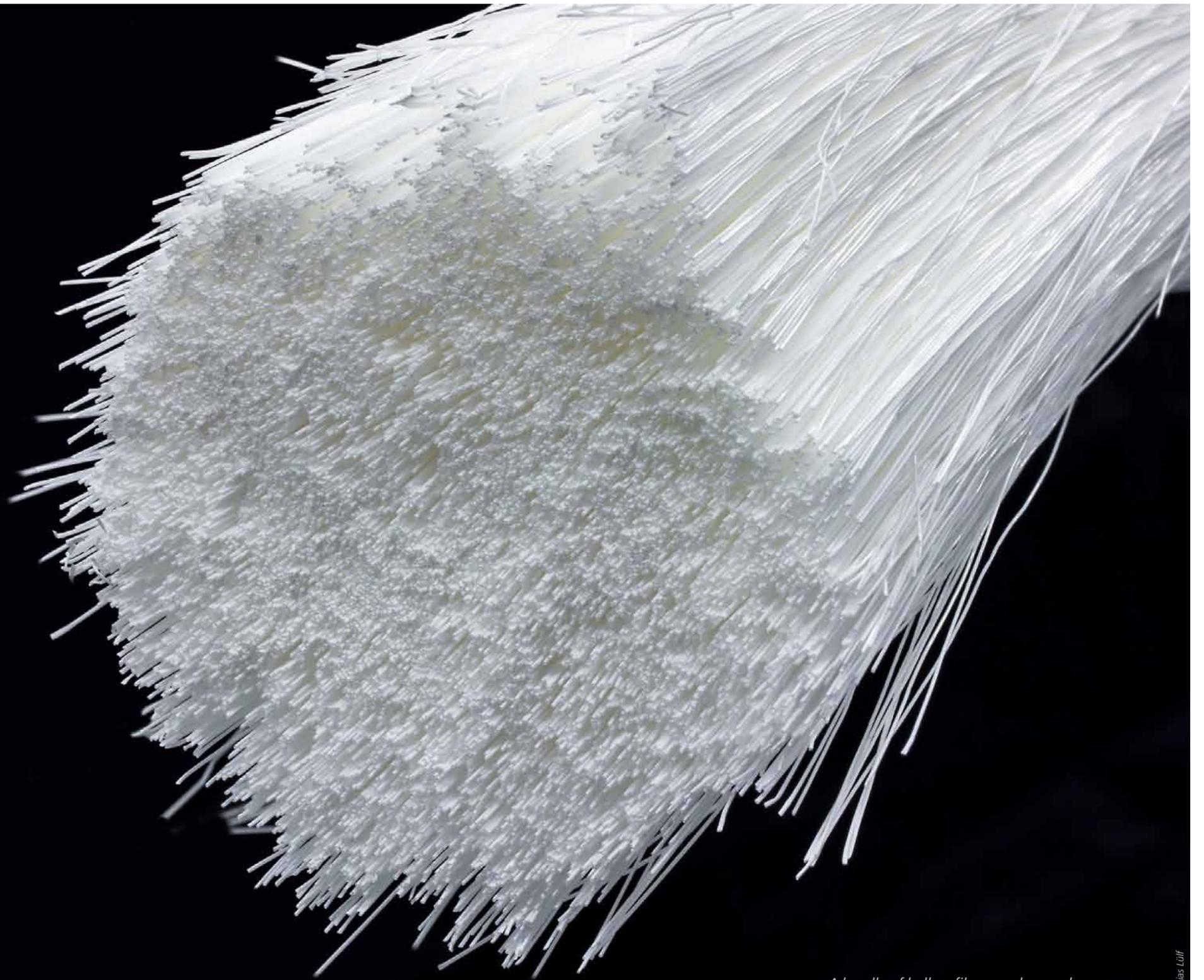
*A bundle of hollow fibre membranes, here ultrafiltration membranes made of polymer.*
