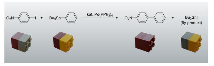
Above: Palladium-catalysed cross-couplings can produce functional materials and bioactive compounds, but at the same time yield unwanted, often toxic by-products (diagram 1). C-H activation makes the production process more environmentally friendly. Below: Electrocatalytic C-H activation can make sustainable use of alternative energy sources, such as wind power (diagram 2).
