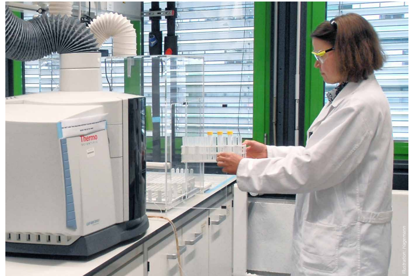
In the lab, metal concentrations are measured using inductively coupled optical emission spectrometry (ICP-OES).
