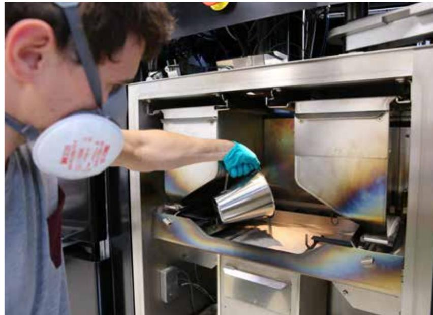
In many additive manufacturing processes, very fine metal powders are fused to form highly complex structures (above). This makes it possible, for example, to create extremely light support structures for aircraft or custom-made implants for a patient (below).
