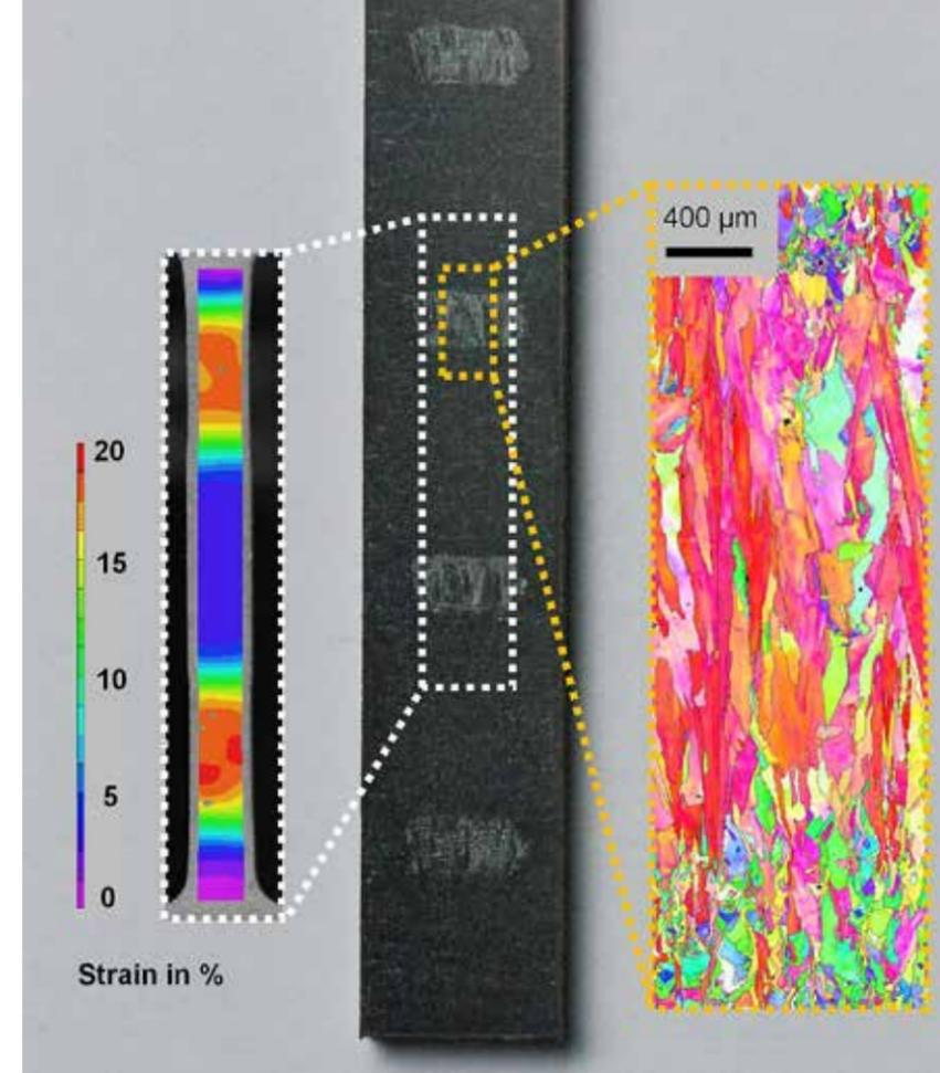
A metal bar (centre) manufactured with different laser sources, featuring multiple transitions between a fine and a coarse microstructure (right). Under loading, greater elongation occurs in areas of the coarse microstructure than in those of the fine microstructure (left).
