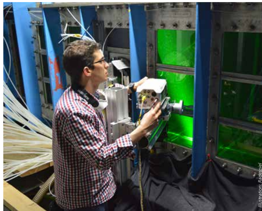
Experiments proving the efficiency of active blowing in the water tunnel at the Technical University of Braunschweig. Optical flow measurement technology methods are used here.
