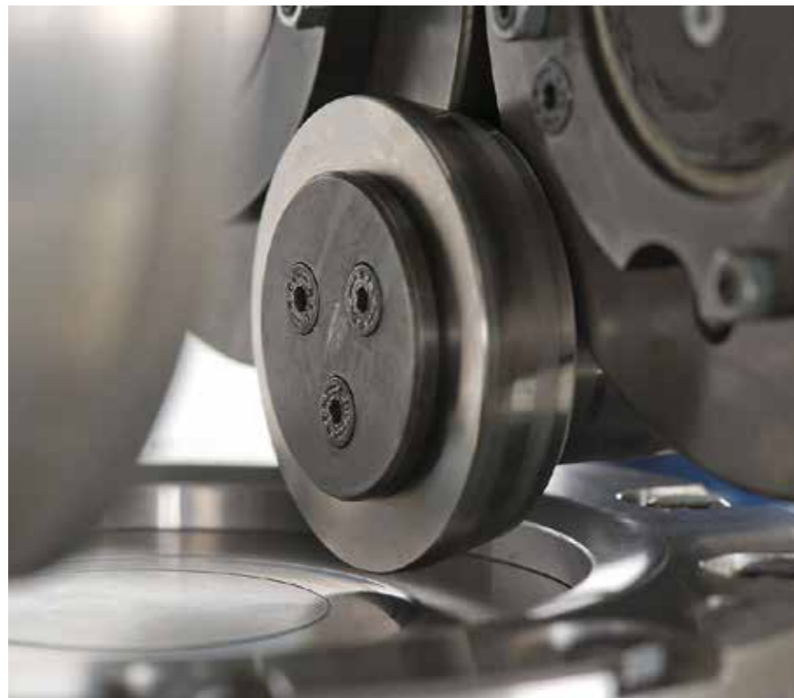
Above: Concentrated work on a flexible rolling system. Below: During rolling, the rotating workpiece is machined such that the material undergoes “process-adapted distribution”. Tool inserts allow a wide range of geometries to be created.
