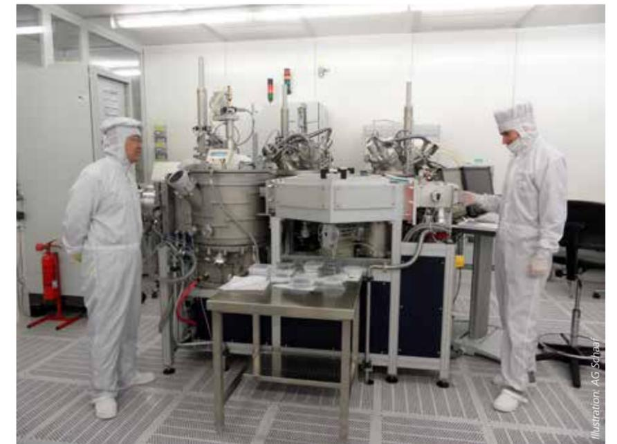
*Researchers must work with nanotechnology under clean room conditions because most dust particles are larger than nanostructures and would interfere. Two researchers working on the “PVD coating plant” in the clean room at the Institute of Micro- and Nanotechnologies at the TU Ilmenau.*
