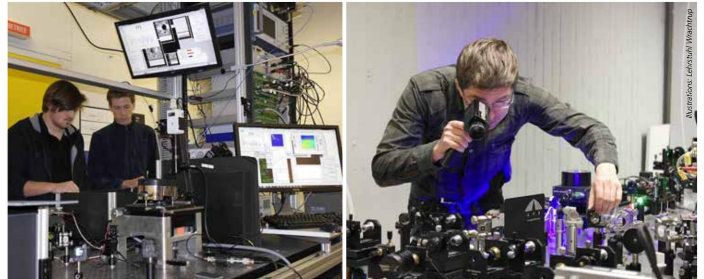
*Above: Doctoral researchers Thomas Häberle and Thomas Öckinghaus working with a diamond magnetometer. Right: Laser spectroscopy is an essential tool in any laboratory where researchers work with diamond defects.*
