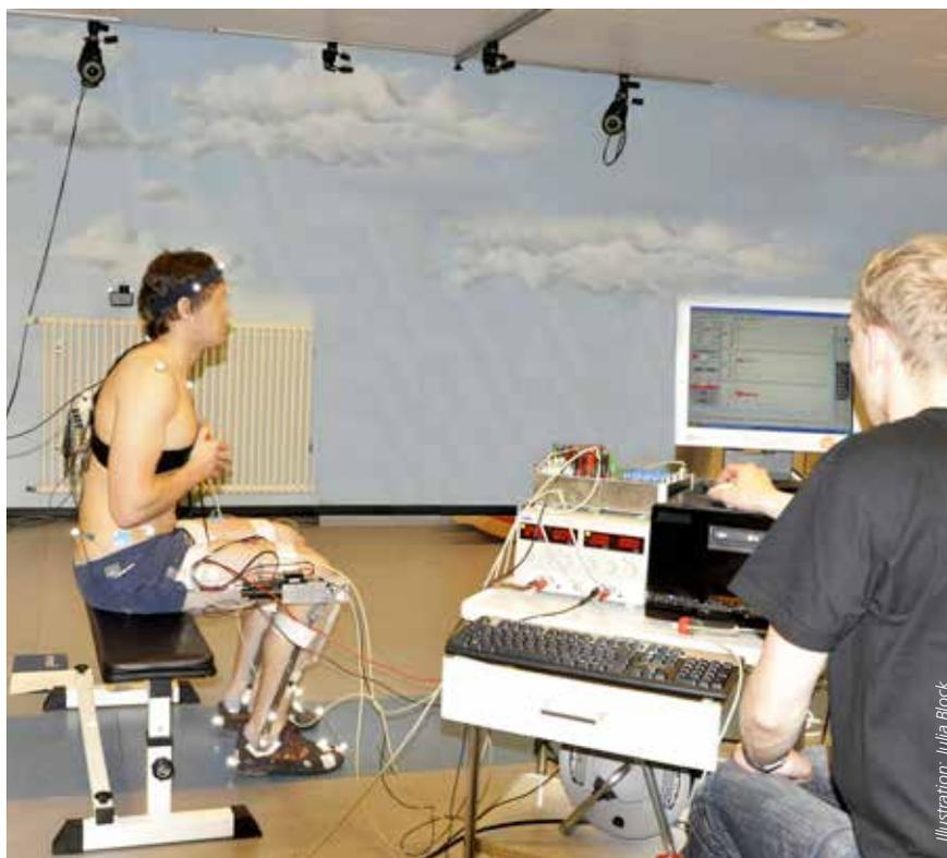
cal model. Force plates embedded in the floor record ground reaction forces under the person's foot. Using these data, it is possible to work out the torques and mechanical forces involved in the motion of the joints.
