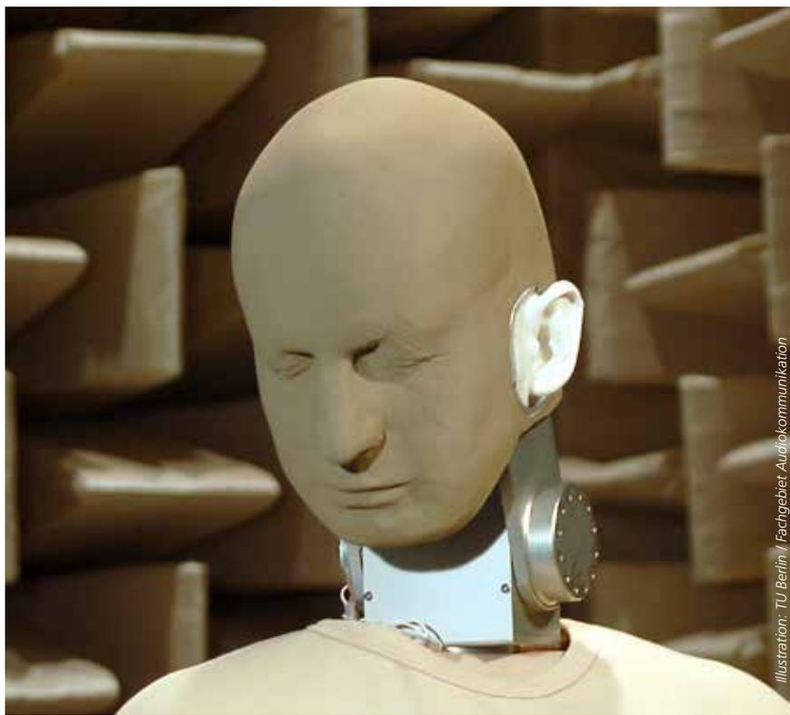
*The binaural robot FABIAN's head movements are controlled by computer. Microphones fitted in the auditory canals of the robot's ears record the acoustic signature of the room.*
