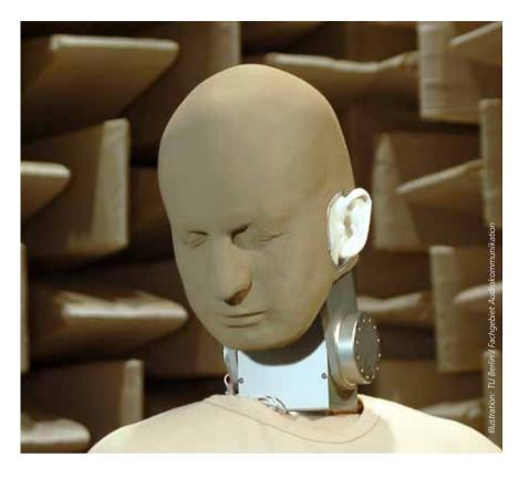
The binarual robot FABIAN's head movements are controlled by computer. Microphones fitted in the auditory canals of the robot's ears record the acoustic signature of the room.
