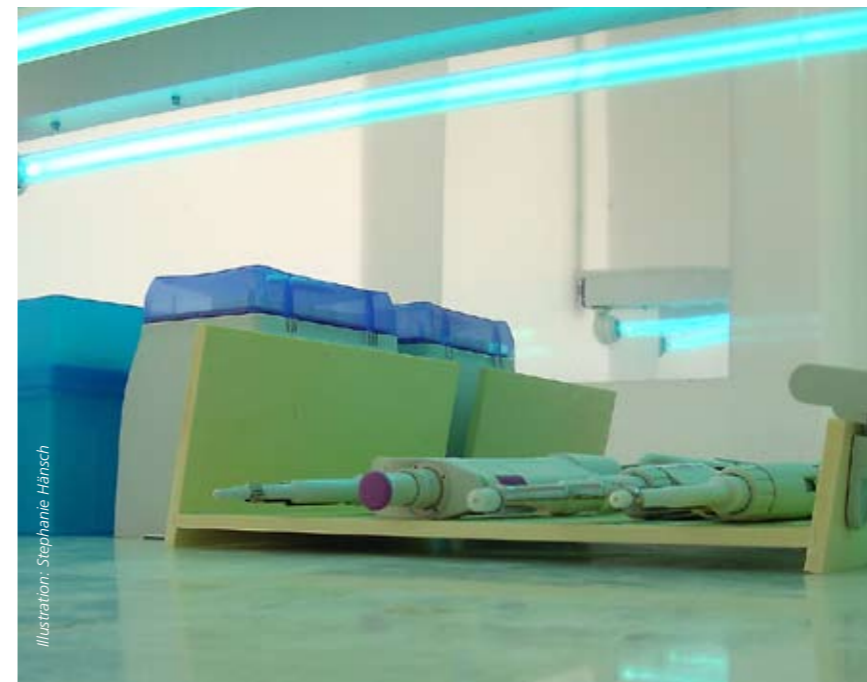
Laboratory instruments are exposed to UV light to destroy foreign DNA molecules.
