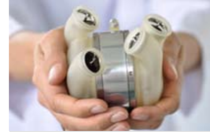
Cover: AME – RWTH Aachen New hope for people suffering from life-threatening heart disease? The Rein-Heart, an artificial heart, has two pump chambers with inlet and outlet valves as well as an electro-mechanical drive.
