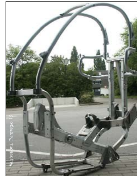
A lightweight frame with the frame structure of the BMW C 1. The covered scooter was launched on the market in the year 2000.
