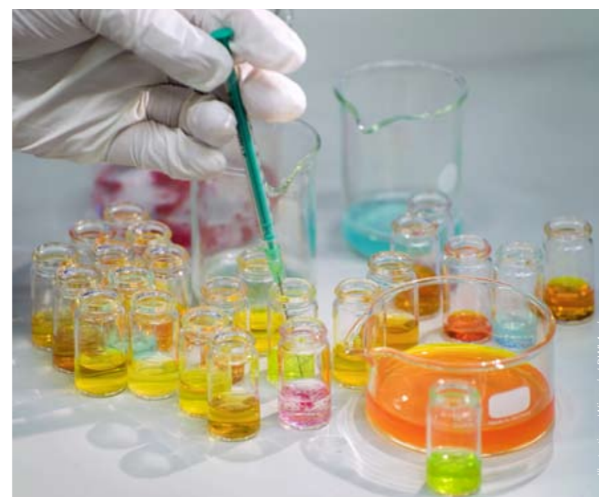
Left: Working with an atomic force microscope. Top: Solutions with light-sensitive sulphonic acid molecules that change their three-dimensional structure on exposure to light.
