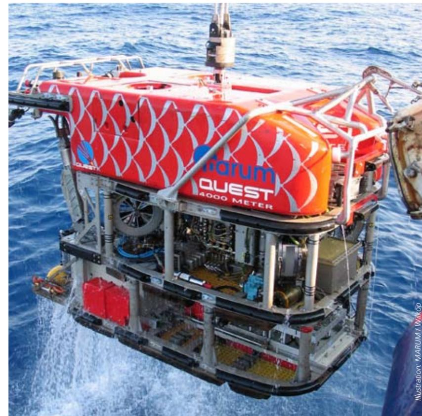
*Power pack in action (top): The deep-sea robot “Quest 4000” of the Bremen cluster of excellence MARUM. Bottom: Using a manipulator arm, the robot collects numerous asphalt samples from the bottom of the Gulf of Mexico, which are examined later in laboratories.*
