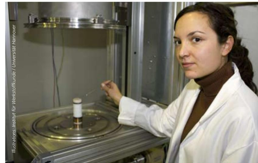
The metal-capillary pressure casting system is used to cast new microcomponents.
