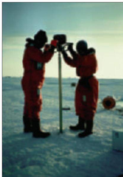
Using motor-driven drills, scientists can obtain ice cores 10 centimetres in diameter. Right: Polar organisms are studied in a refrigerated container on board the "Polarstern".
