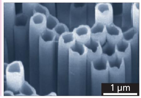
In the final step of this process, the template fibre is removed. One way to achieve this is to raise the temperature of the material, in order to decompose the polymer into easily volatised building blocks. As an alternative, the fibres can also be removed with a solvent or, with suitable types of fibres, by using biological degradation.
