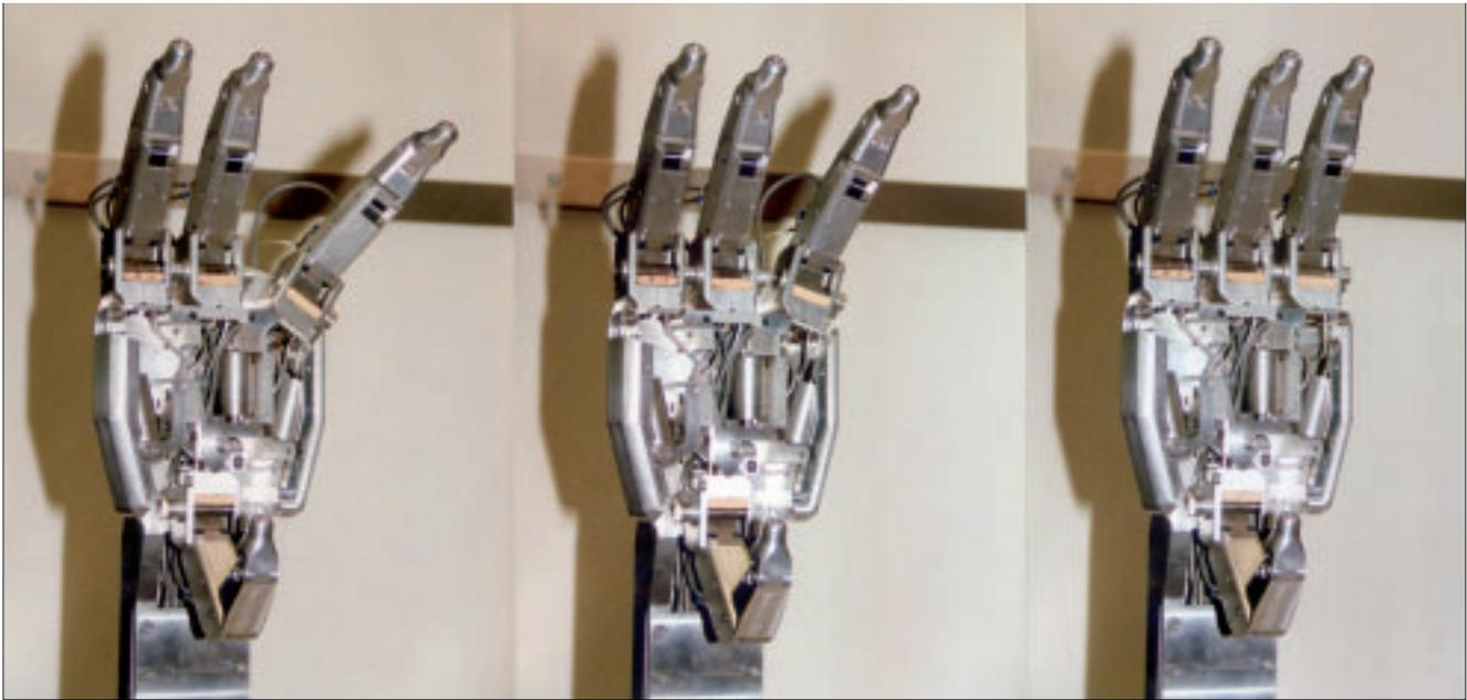
The palm of the "Aachen-IFAS-Hand" contains three cylinder-lever drives. They allow the thumb and the two outer fingers to move parallel to the palm. The piston rod is connected to one end of the proximal joint (the one nearest the hand) and the lever end is connected to the other end and to the back of the hand.
