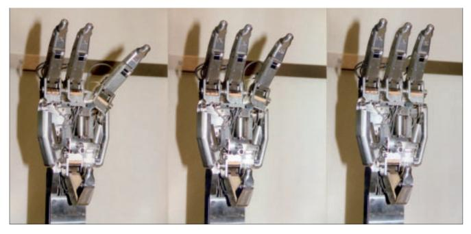
The palm of the "Aachen-IFAS-Hand" contains three cylinder-lever drives. They allow the thumb and the two outer fingers to move parallel to the palm. The piston rod is connected to one end of the proximal joint (the one nearest the hand) and the lever end is connected to the other end and to the back of the hand.
