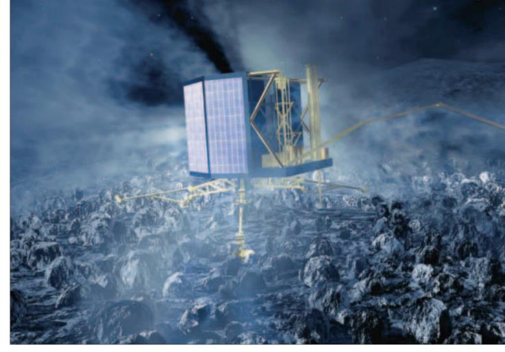
After landing, harpoons need to be launched to anchor the lander because the comet has almost no gravitational force. A drill will be used to take rock and soil samples and data will be transmitted to the ESA's satellite control centre in Darmstadt via an antenna.
