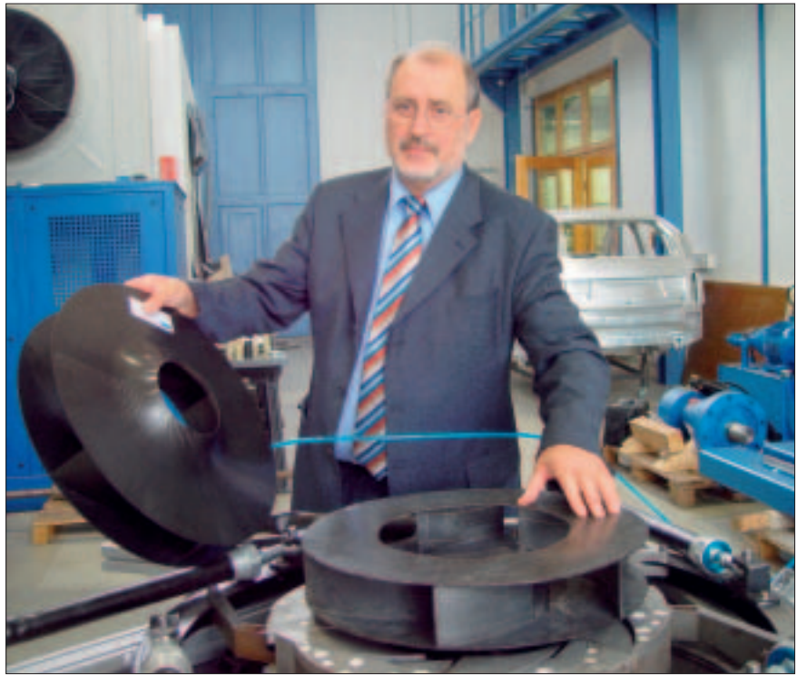
Textile fabrics made of carbon fibres and thermoplasts form the basis of the new rotor. Above: The elastic preform is clamped and baked in an autoclave, a special oven, to produce the final high-performance rotor.
