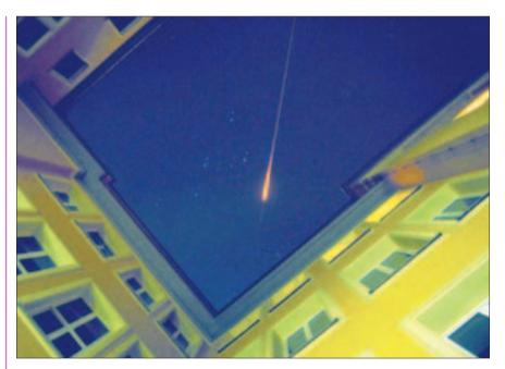
Left: A spectacle of nature – jagged lightning cuts through the sky. Above: An artificial bolt of lightning in the evening sky: High-power pulses of laser light generate a long, white ray of light (a plasma focus) shining in the sky. This picture was taken from the courtyard of the Department of Physics at the University of Jena.
