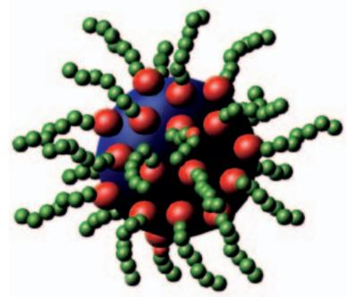
Ferrofluids contain minute magnetic particles that have a diameter of only ten nanometres. These nanoparticles can be coated with long-chain molecules (shown here in green). The surface coating is not shown to scale in the modelled particle for reasons of clarity.
