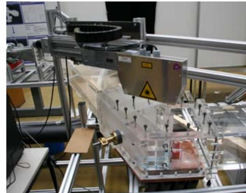
Left: Laboratory setup used for highly precise measurements of the ice layer thickness with a light-stripe sensor. Bottom: The laser stripe is clearly visible on the ice contour.
