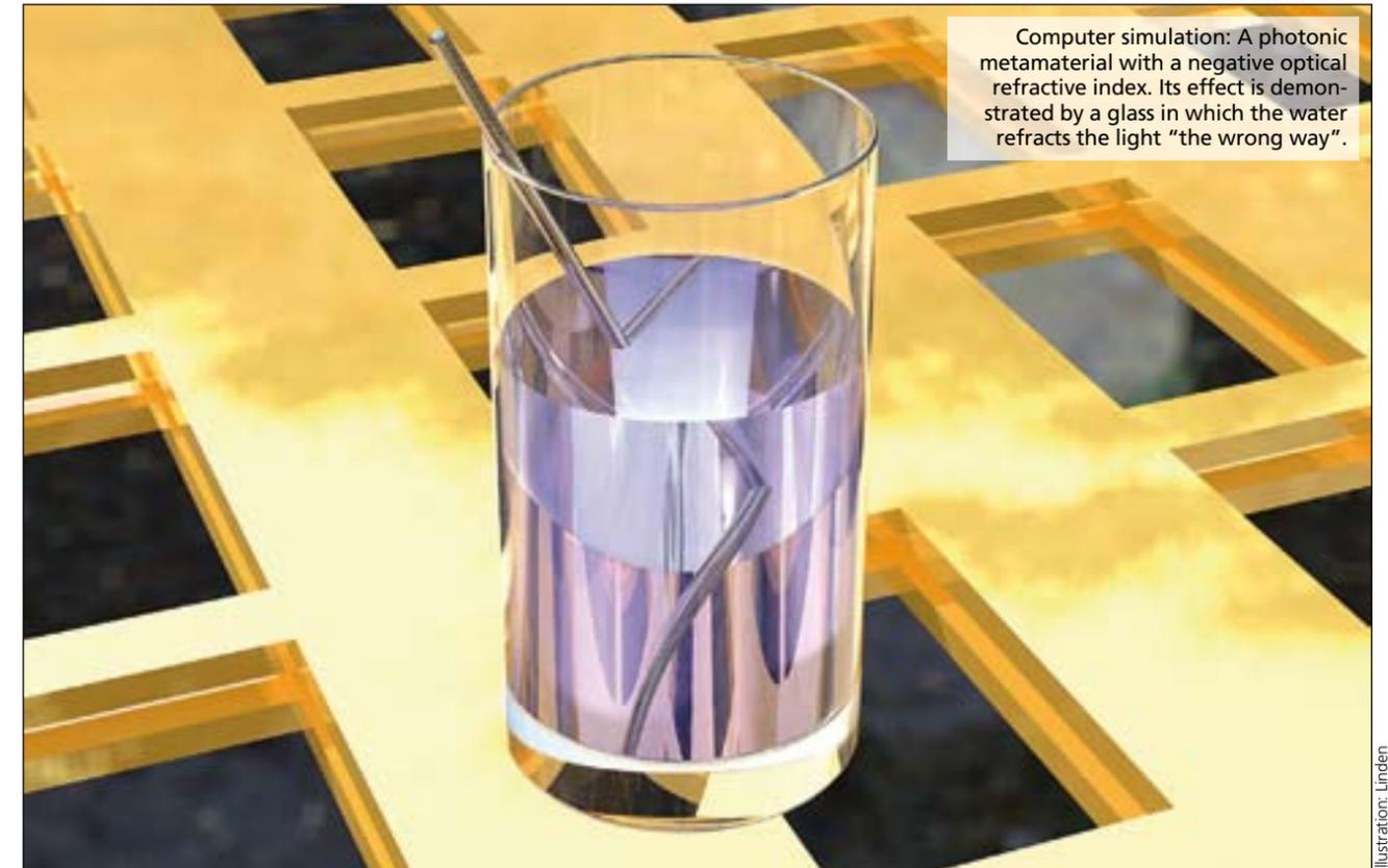
Computer simulation: A photonic metamaterial with a negative optical refractive index. Its effect is demonstrated by a glass in which the water refracts the light "the wrong way".
