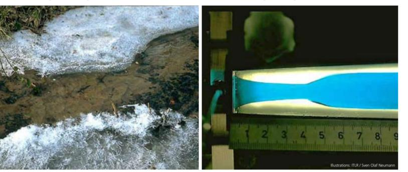
Left: A small brook with characteristic ice deposits along the edges. Right: Formation of ice (white) in a flow channel. Nature on the left, technology on the right – the similarity between the two structures is clearly apparent.
