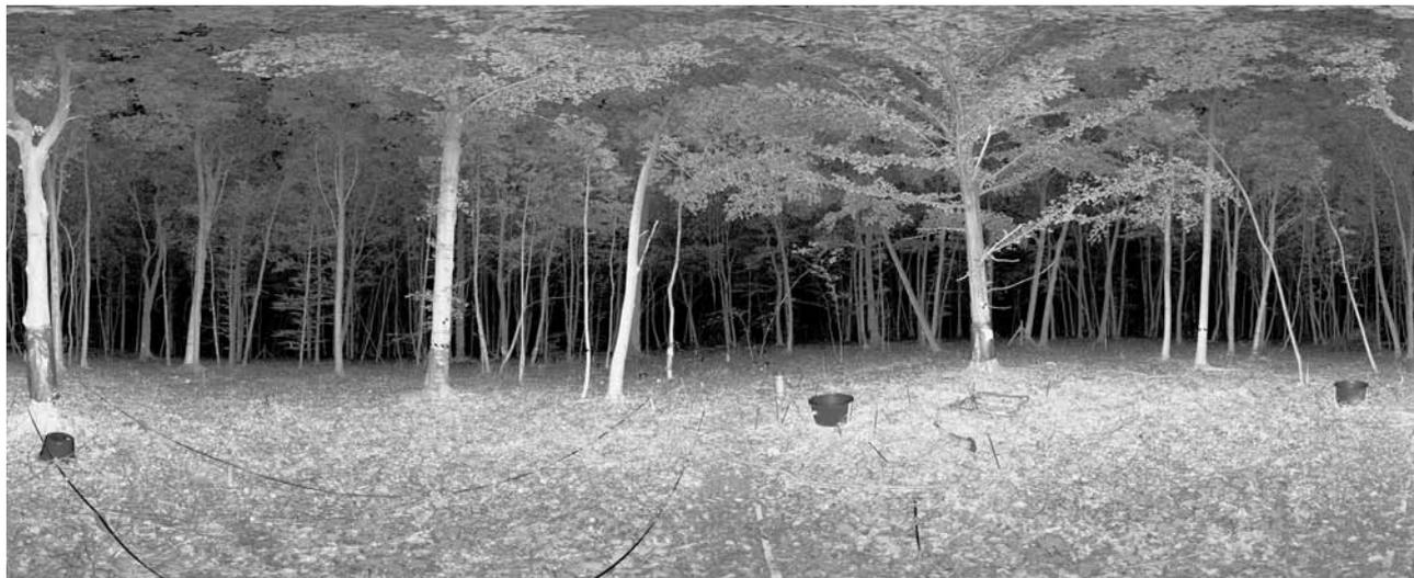
*Using 3D scans such as this one, the researchers can create three-dimensional maps of the forests, showing structural information that provides the basis for combined quantitative analysis of data in ecosystem models.*
