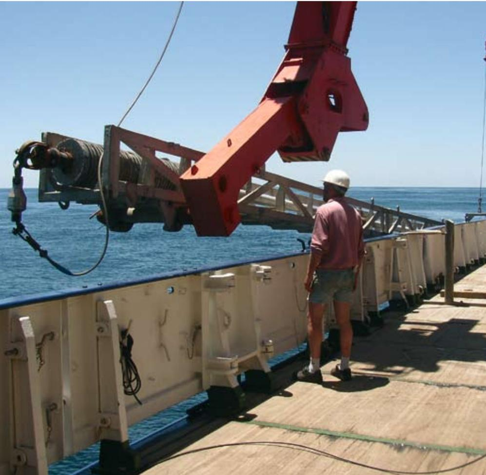
*On board the research vessel Meteor: Gravity cores are won from the seabed.*
