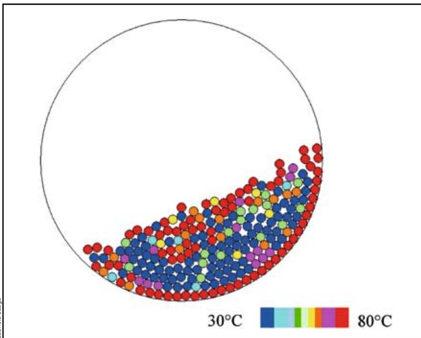
2D simulation of the heat transmission in mechanically mixed bulk material: temperature distribution in the bulk material.
