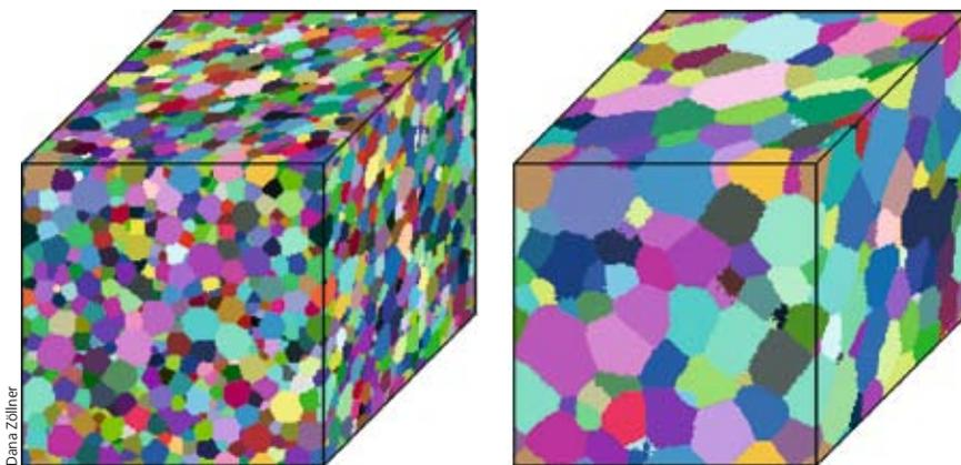
With a modified Monte Carlo algorithm Dana Zöllner succeeds in simulating the growth of a crystalline micro-structure in three dimensions.
