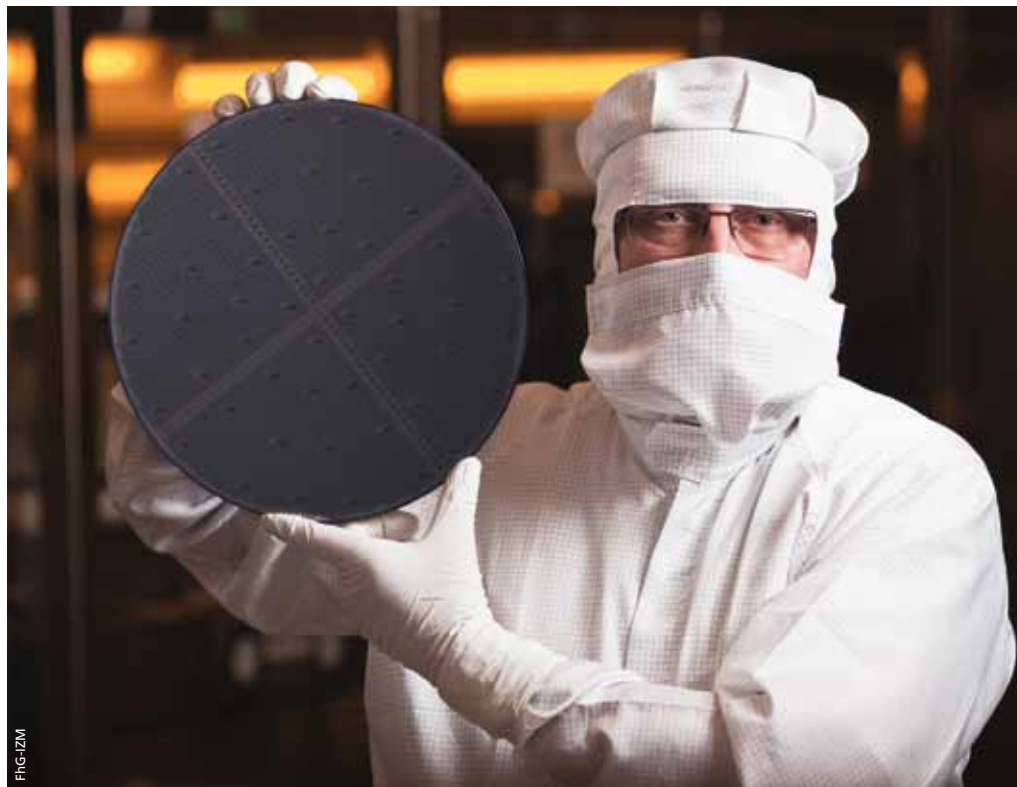
As the wafers from semiconductor material for chip production continue to increase in size — several hundred microchips fit on this 300-mm wafer — the structures in the chips themselves are becoming smaller and smaller. The reliable wiring of up to a billion transistors on a single chip is the subject of the International Research Training Group 1215.
